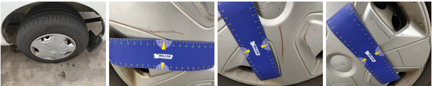
Wheel Rear Left / Wheel Cover / Replace-scratch
