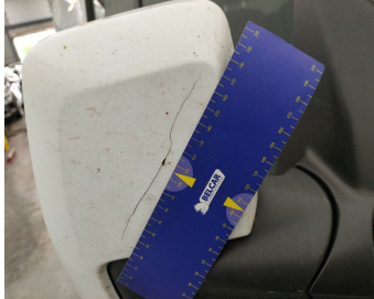
Side View Mirror Right / Shell / Replace Painted-cracked
