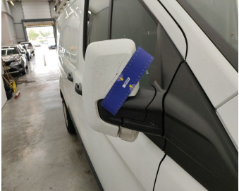
Side View Mirror Right / Shell / Replace Painted-cracked
