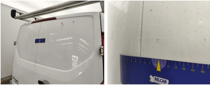
Rear Loading Door Right // Repair & Painting-scratch
