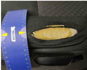
Seat Front Left / Bottom Coating / Replace-hole
