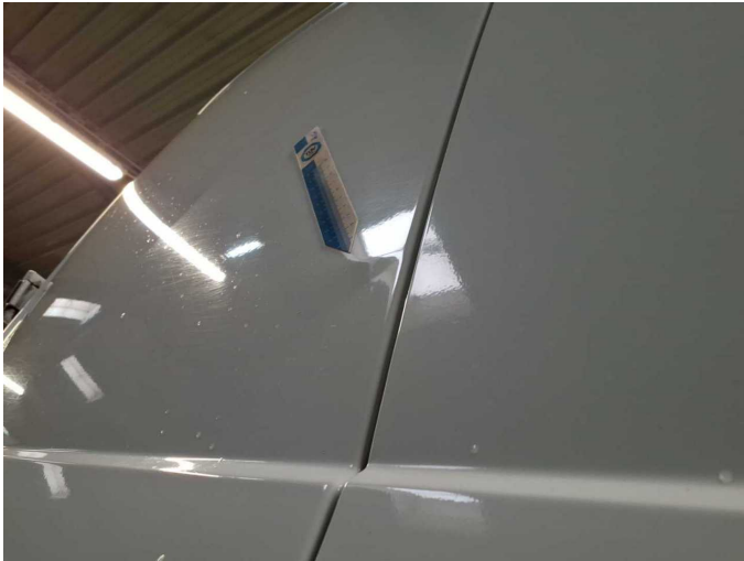
Damage 4: Boot lid / rear door: Rear door - left side - Deformed - Loss in value
