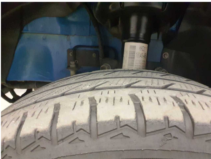
Damage 3: Wheel / tyres: Tyre - front (unter 4mm) - Worn - Replace
