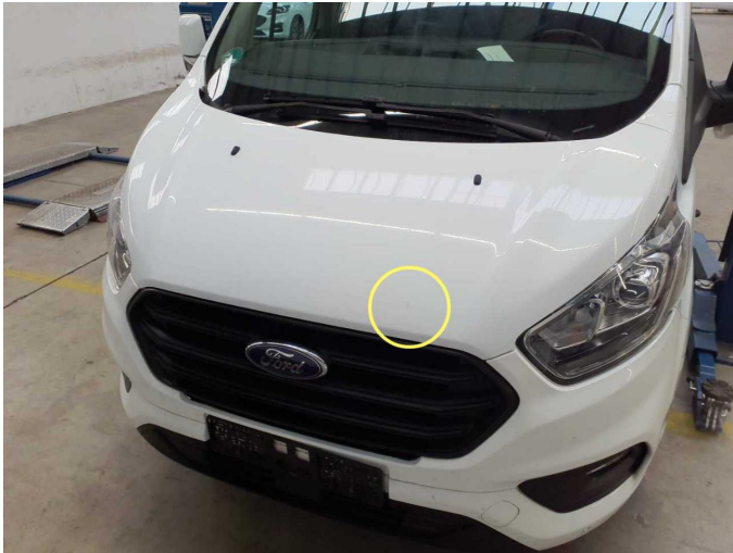
Damage 3: Bonnet: Bonnet - dent(s) - Smooth repair work
