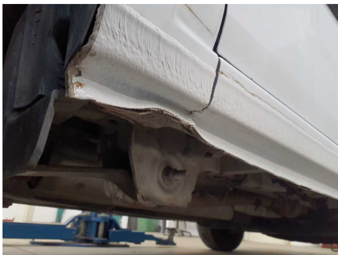
Damage 7: Sill - right side: Sill - Damaged - Repair and paint
