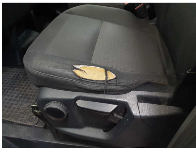
Damage 8: Seat - front: Seat cover - left side - Damaged - Replace
