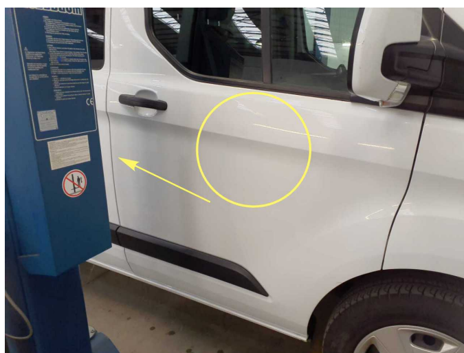
Damage 10: Door - front right side: Door edge - Dent / paintcoat damage - Repair and paint
