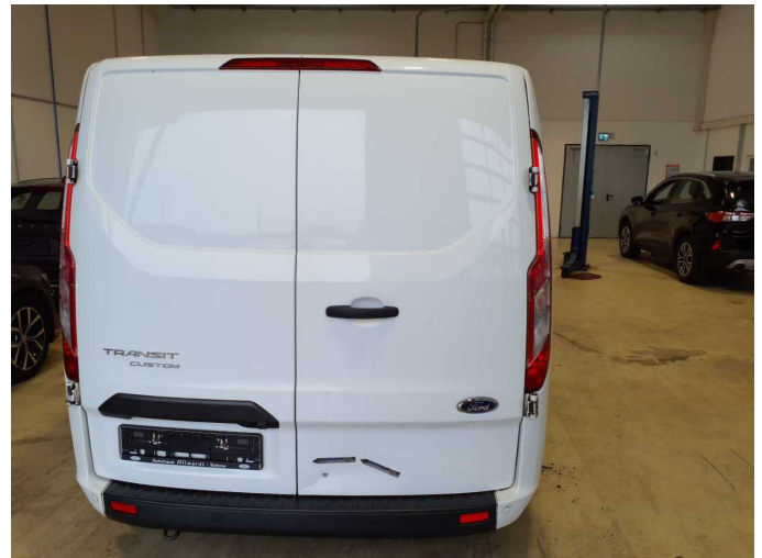
Damage 4: Boot lid / rear door: Rear door - right side - Deformed - Repair and paint
