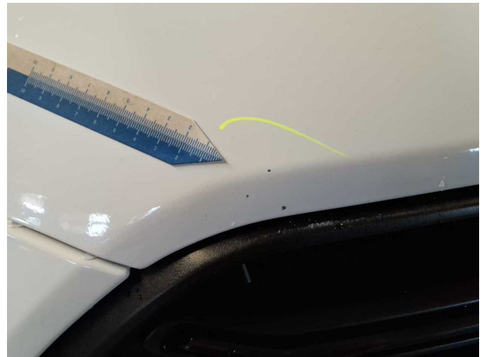
Damage 7: Bonnet: Bonnet - Stone chips - Paint
