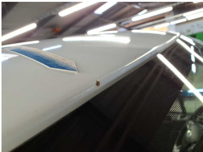
Damage 8: Roof: Roof - Corrosion - Paint
