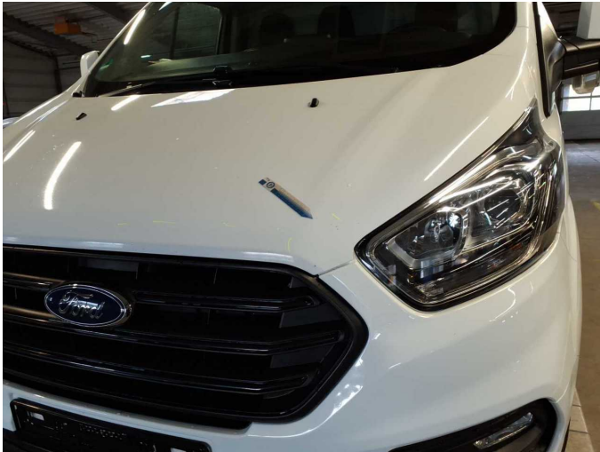
Damage 7: Bonnet: Bonnet - Stone chips - Paint
