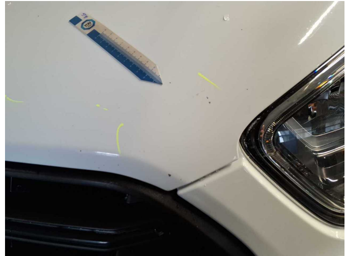
Damage 7: Bonnet: Bonnet - Stone chips - Paint
