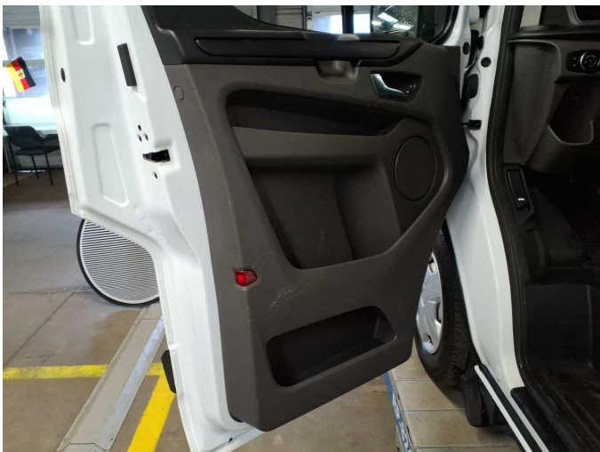
Damage 6: Trim / covers: Door trim - front left side - Scratch(es) - Replace
