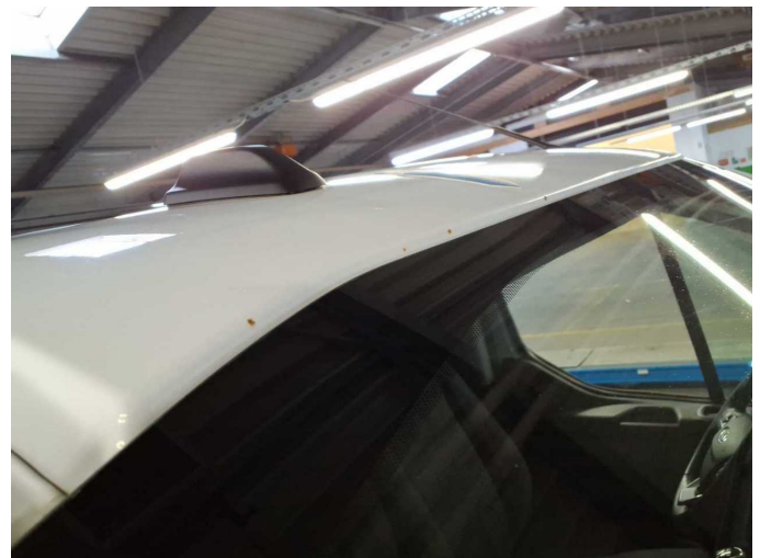
Damage 8: Roof: Roof - Corrosion - Paint
