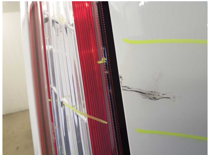
Damage 5: Tail light: Tail lamp - left side - Scratch(es) - Replace
