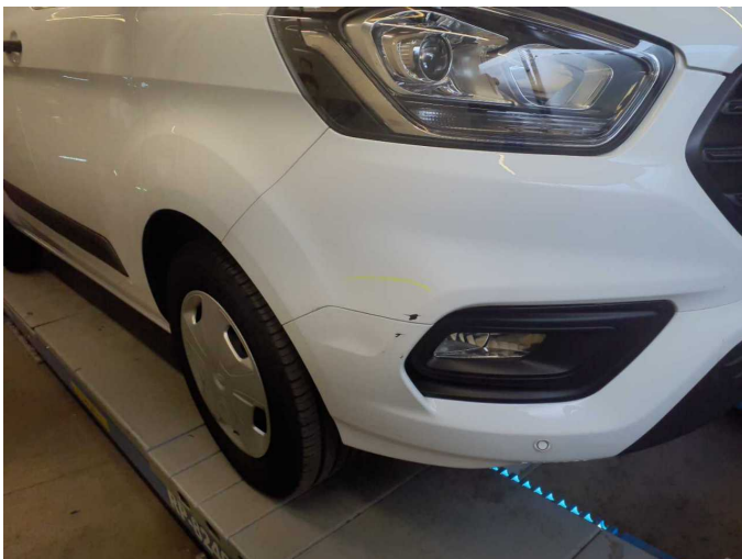
Damage 6: Front bumper: Front bumper - Scratch(es) - Paint
