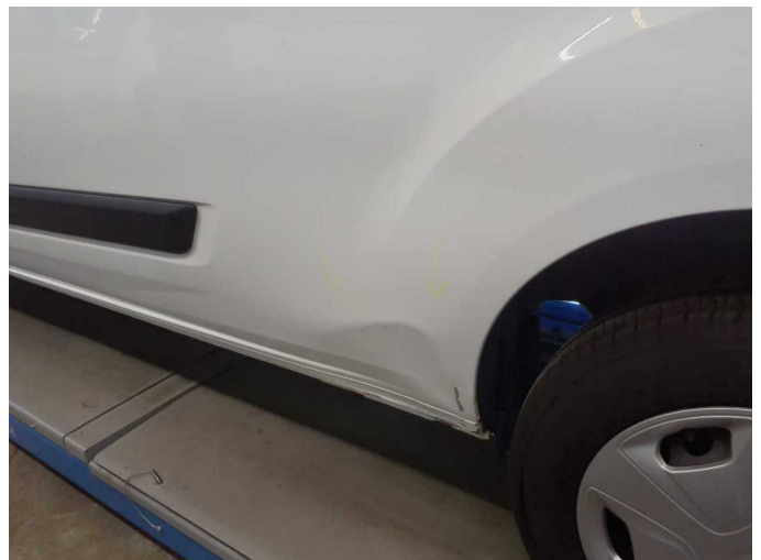
Damage 7: Sill - left side: Sill (/Seitenwand) - Deformed - Repair and paint
