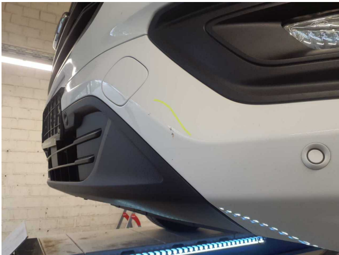
Damage 6: Front bumper: Front bumper - Scratch(es) - Paint
