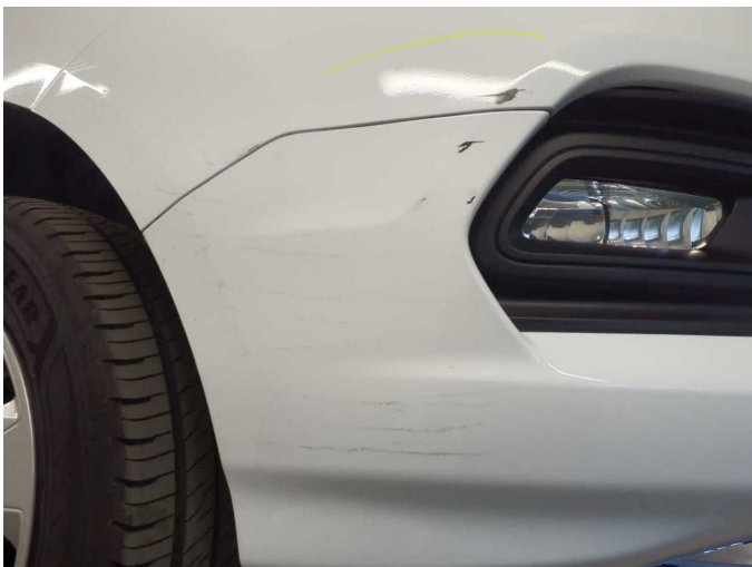
Damage 6: Front bumper: Front bumper - Scratch(es) - Paint
