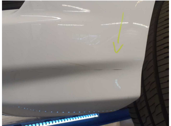
Damage 6: Front bumper: Front bumper - Scratch(es) - Paint
