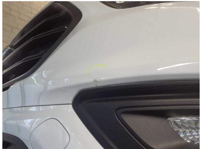
Damage 6: Front bumper: Front bumper - Scratch(es) - Paint
