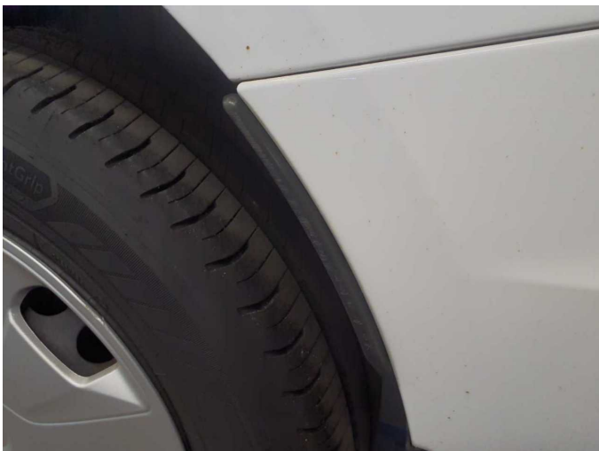
Damage 2: Side panel - rear left side: Mud flap - Scratched - Replace
