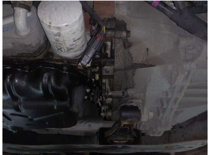
Damage 4: Engine: Engine (/getriebe) - Leaking - Perform diagnosis
