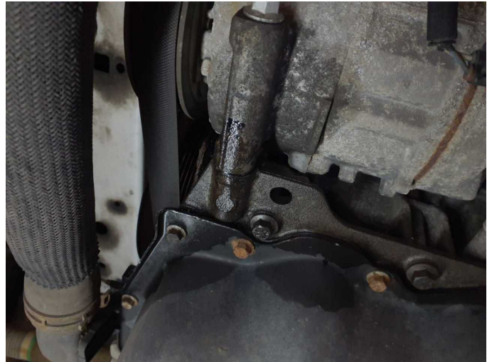
Damage 5: Engine: Engine - Leaking - Perform diagnosis
