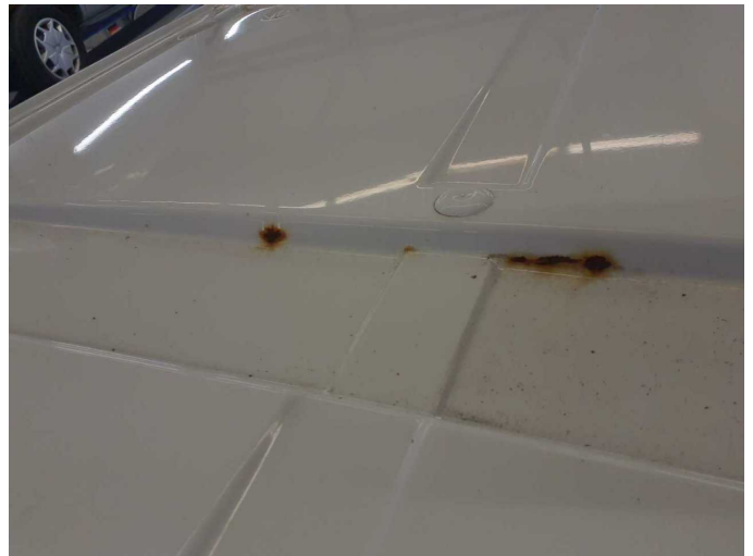
Damage 8: Roof: Roof - Corrosion - Smart repair
