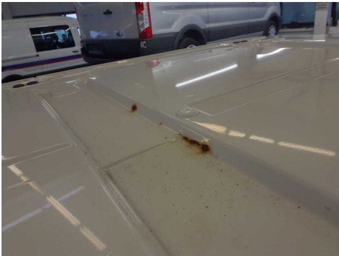
Damage 8: Roof: Roof - Corrosion - Smart repair
