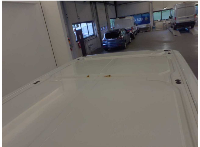
Damage 8: Roof: Roof - Corrosion - Smart repair
