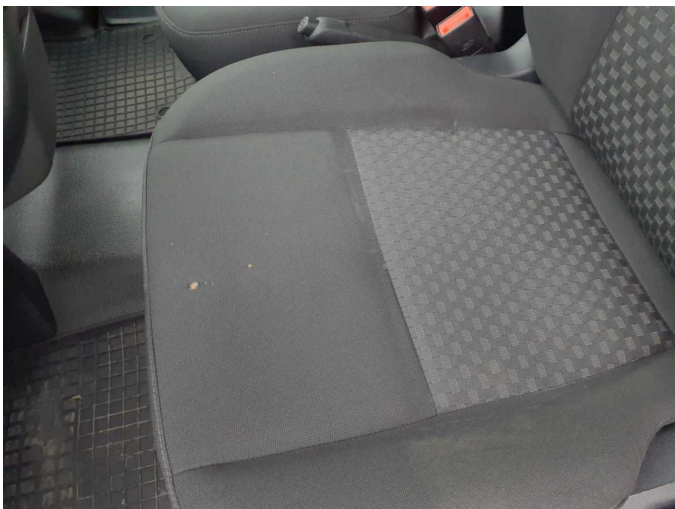
Damage 9: Seat - front: Seat cover - left side - Holes - Replace
