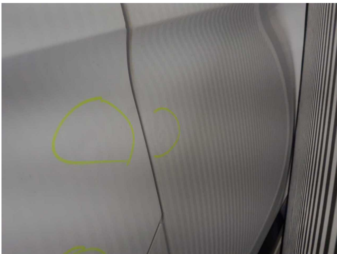
Damage 1: Side panel - rear left side: Side panel (1) - dent(s) - Smart repair
