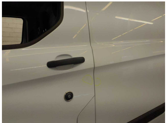
Damage 2: Door - front left side: Door (2) - dent(s) - Smart repair
