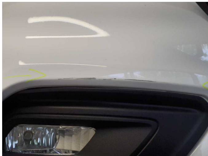
Damage 6: Front bumper: Front bumper - Scratch(es) - Paint
