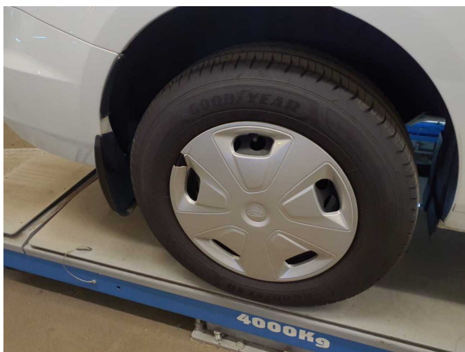
Damage 1: Wheel / tyres: Wheel cover - rear right side - Broken / torn - Replace
