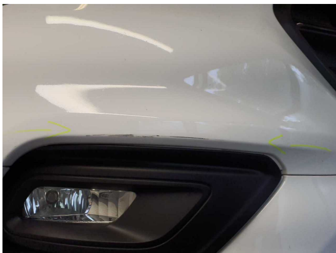
Damage 6: Front bumper: Front bumper - Scratch(es) - Paint
