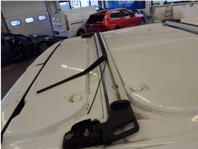
Damage 2: Equipment: Roof rack system (Dichtung hintere schiene) - Broken / torn - Replace
