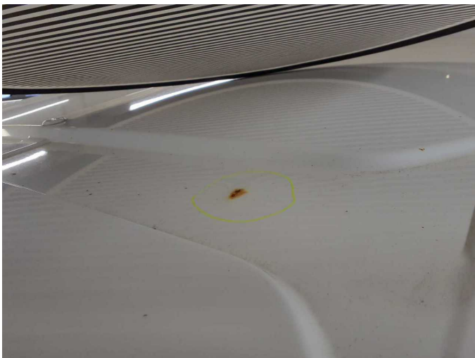
Damage 4: Roof: Roof (+Beule) - Corrosion - Smart repair
