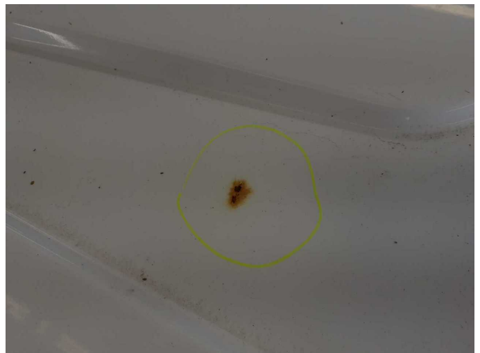
Damage 4: Roof: Roof (+Beule) - Corrosion - Smart repair
