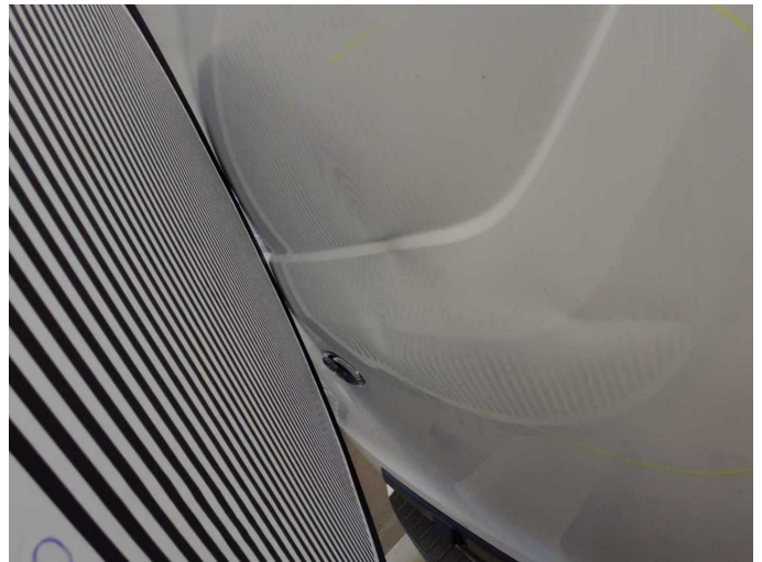
Damage 5: Boot lid / rear door: Boot lid - Deformed - repair according to calculation
