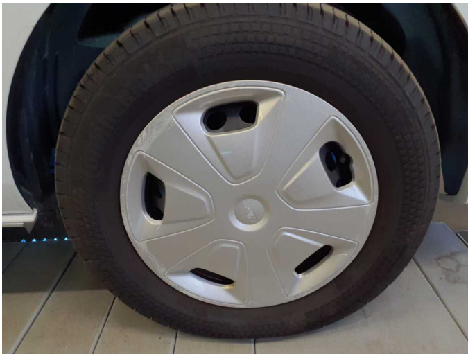
Damage 1: Wheel / tyres: Wheel cover - front right side - Scratched - Replace
