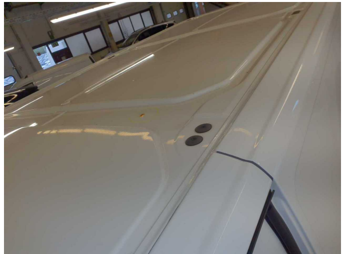
Damage 4: Roof: Roof (+Beule) - Corrosion - Smart repair
