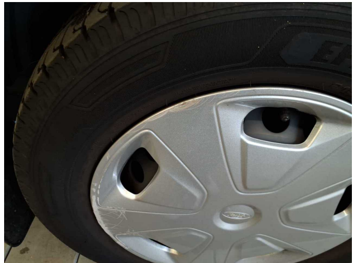
Damage 2: Wheel / tyres: Wheel cover - front right side - Scratch(es) - Replace
