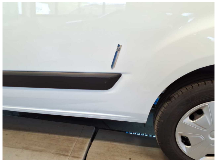
Damage 4: Side panel - rear left side: Brightware - Scratch(es) - Replace
