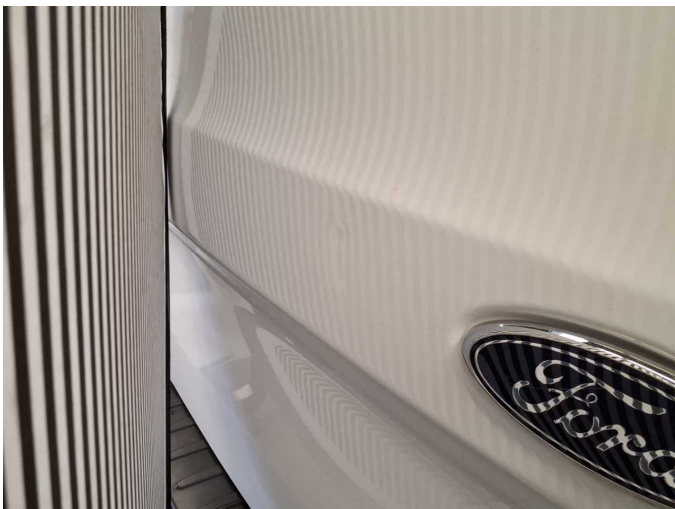
Damage 6: Boot lid / rear door: Boot lid (Rechts) - Deformed - Repair and paint
