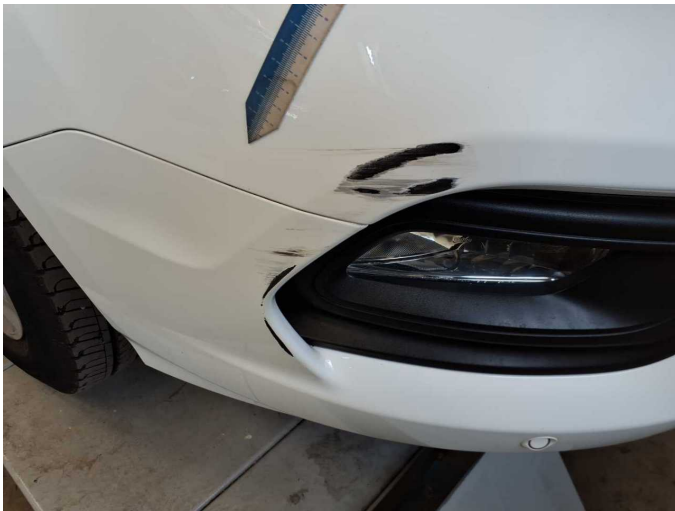
Damage 5: Front bumper: Front bumper - Scratch(es) - Paint
