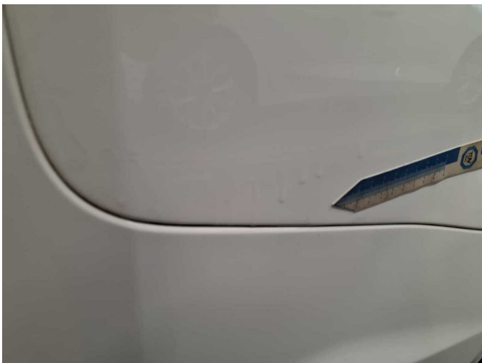
Damage 8: Side panel - rear right side: Side panel (Lackläufer) - Unprofessionally repaired - Repair and paint
