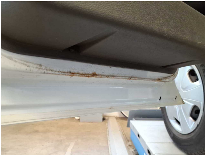
Damage 7: Door - front left side: Door - Corrosion - Repair and paint
