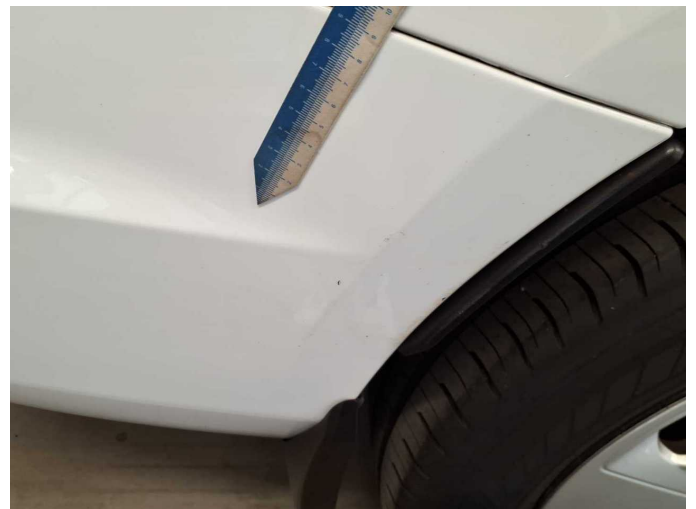
Wear and tear 3: Rear bumper: Bumper - rear right side - Scratch(es) - No deduction
