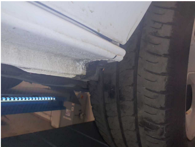
Damage 2: Mudguard - right side: Mud flap - Broken / torn - Replace
