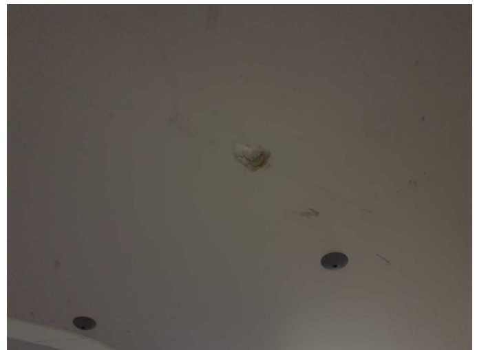
Damage 3: Trim / covers: Boot lid - interior trim - Broken / torn - Replace
