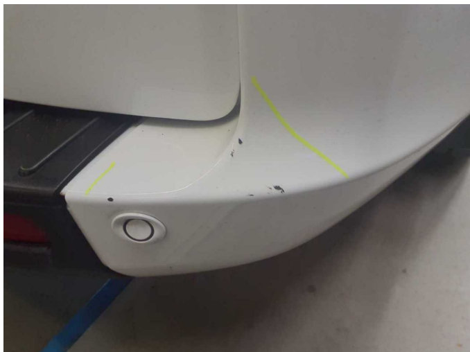
Damage 5: Rear bumper: Bumper - rear right side - Scratch(es) - Paint
