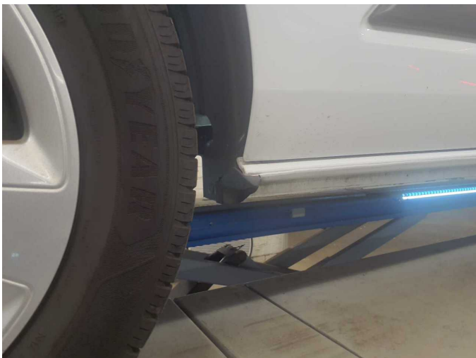
Damage 1: Mudguard - left side: Mud flap - Broken / torn - Replace
