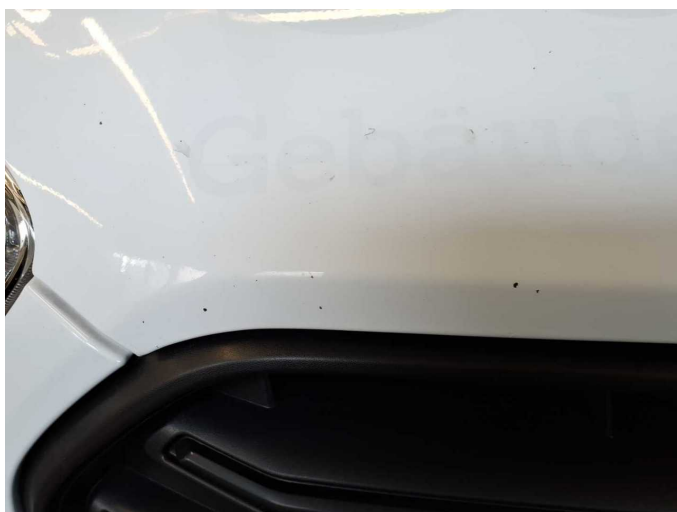
Damage 7: Bonnet: Bonnet - Stone chips - Paint
