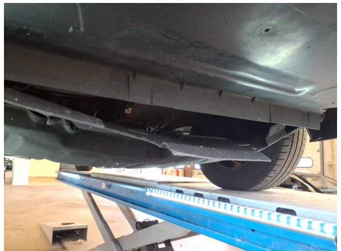
Damage 4: Body: Underbody panelling - Malposition - Repair
