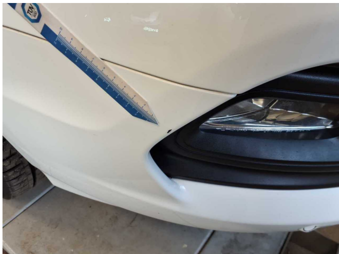
Damage 8: Front bumper: Front bumper (unterhalb) - Scratch(es) - Paint
