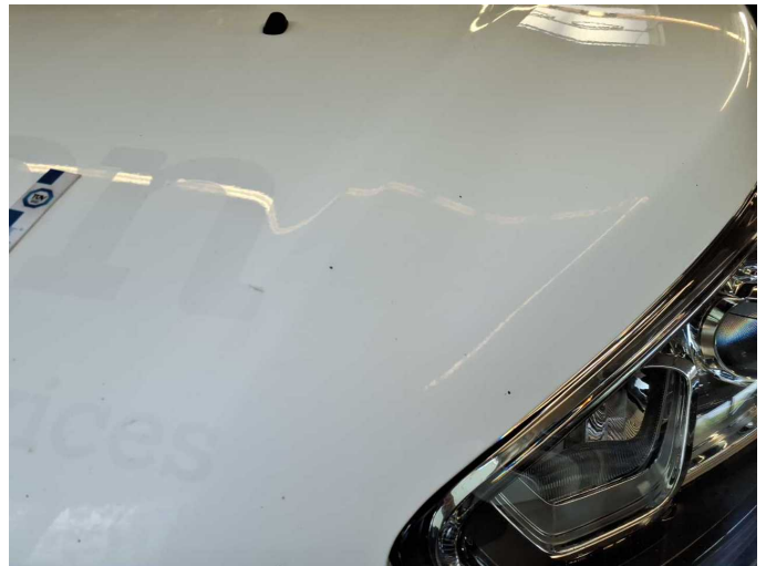
Damage 7: Bonnet: Bonnet - Stone chips - Paint
