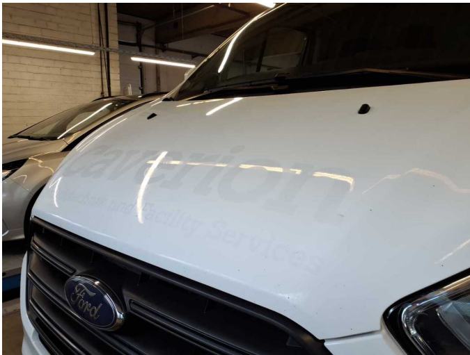
Damage 6: Body: Body (Klebereste) - Glued / labelled - De-glue / neutralise
