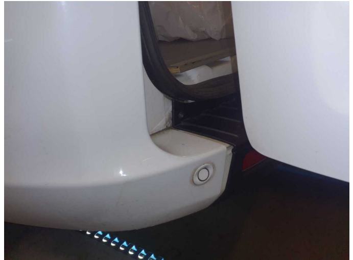
Damage 1: Rear bumper: Rear bumper - Malposition - Un- / install
