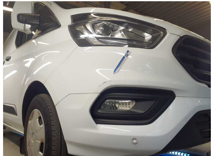
Damage 5: Front bumper: Front bumper - Scratch(es) - Paint
