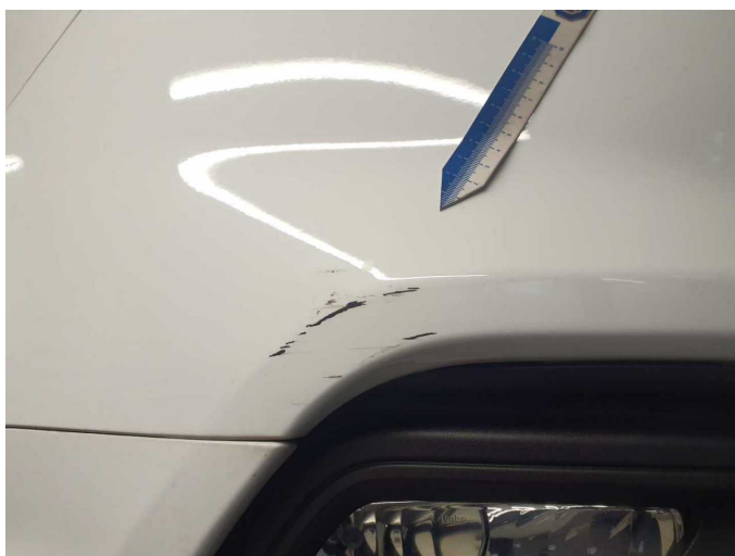
Damage 5: Front bumper: Front bumper - Scratch(es) - Paint
