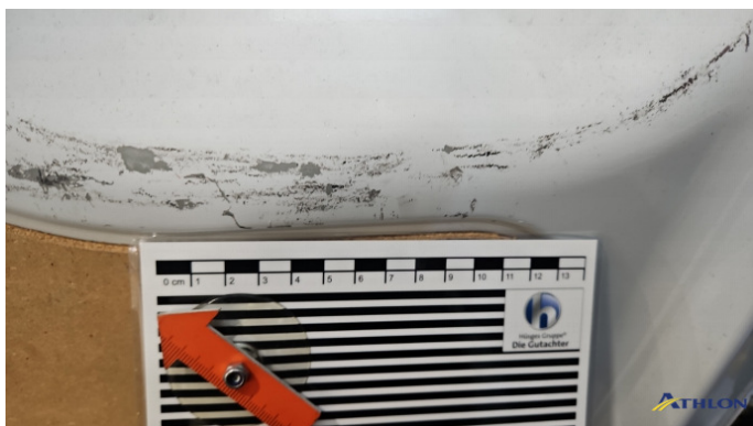
7. Hecktür Links Kratzer Ab 60mm
