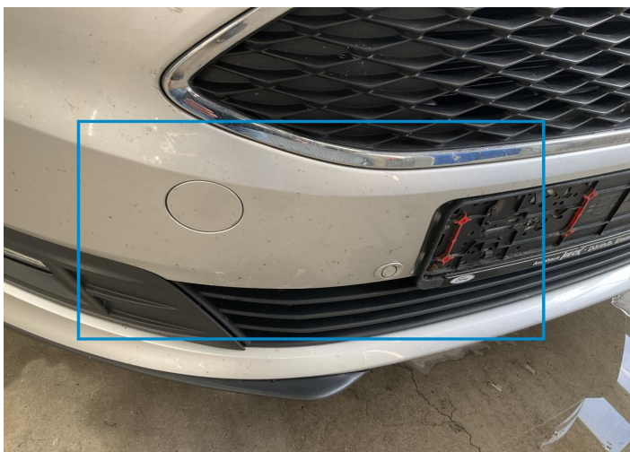
1. Bumper / Front Paint / Scratch / Scuff -
