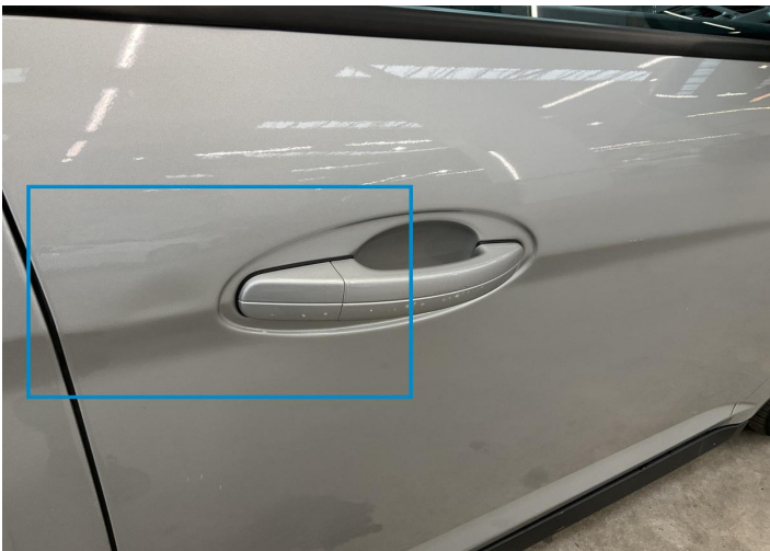
8. Door / Front Right Bodywork / Dent / Dent -
