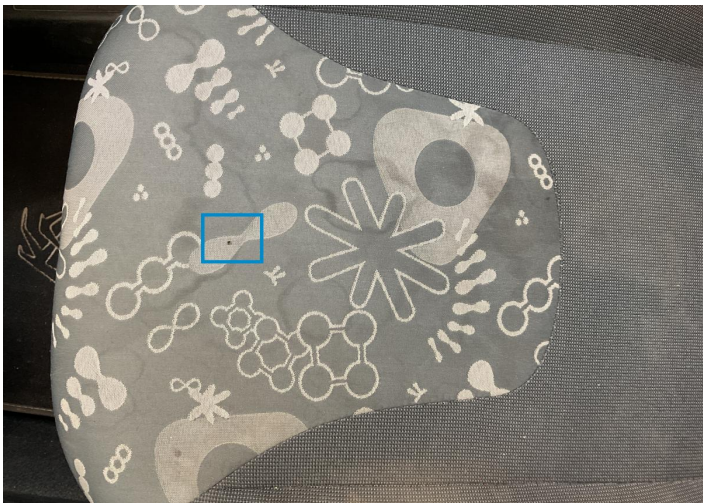
1. Seat Cushion / Front Right Interior / Burn -
