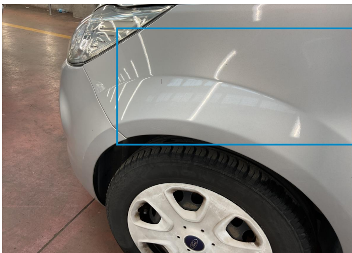
13. Fender / Front Left Bodywork / Poor Previous Repair -
