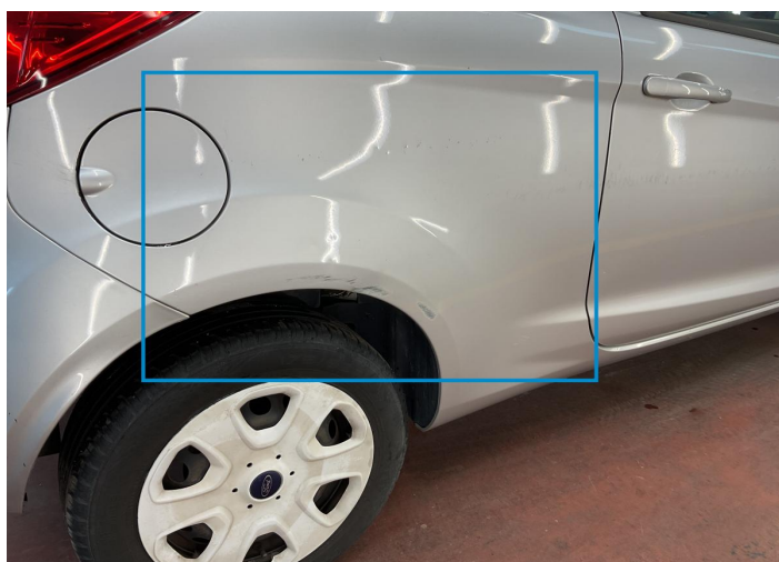
21. Fender / Back Right Bodywork / Dent -
