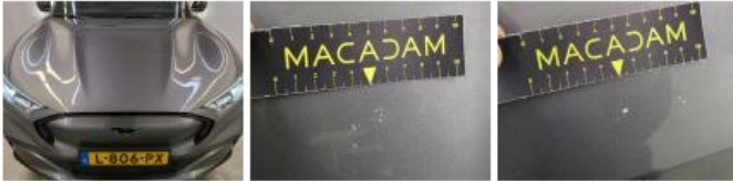
Wing RR, Scratch(es), Repair and paint (complete)
