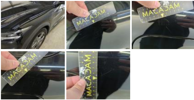
Bonnet, Scratch(es), Repair and paint (complete)
