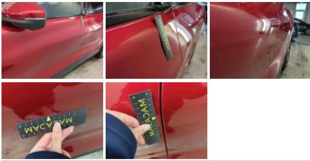
Door RL, Scratch(es), Repair and paint (complete)
