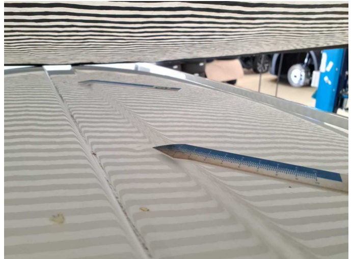
Damage 4: Roof: Roof - dent(s) - Smart repair
