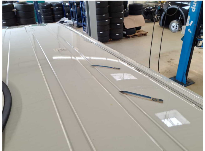
Damage 4: Roof: Roof - dent(s) - Smart repair
