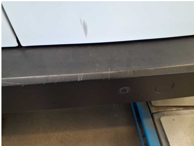
Damage 2: Rear bumper: Rear bumper (unpainted) - Scratch(es) - Loss in value
