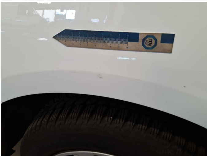
Damage 5: Side panel - rear right side: Side panel (Beule) - Dent / paintcoat damage - Repair and paint
