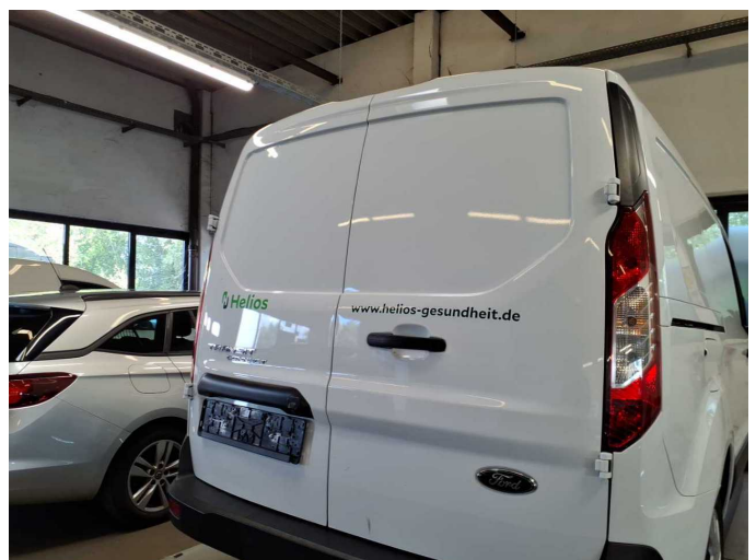
Damage 3: Body: Body - Glued / labelled - De-glue / neutralise
