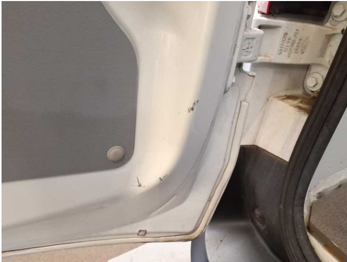
Wear and tear 1: Boot lid / rear door: Boot lid (Links innen) - Scratch(es) - Smart repair
