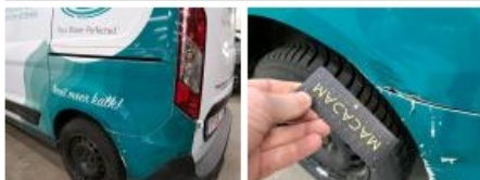
Wheel cover RL, Missing, Replace
