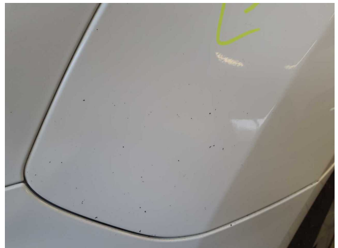
Damage 5: Mudguard - left side: Mudguard - left side (+Steinschläge) - Paint defect - Paint
