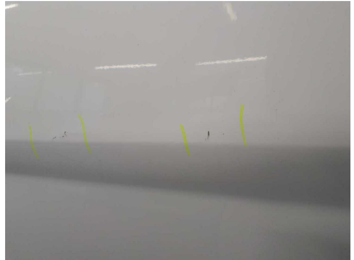
Damage 4: Side panel - rear left side: Side panel (3 Dellen+Kratzer) - Dent / paintcoat damage - Smart repair
