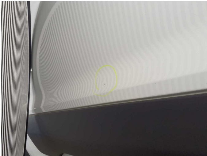
Damage 1: Sliding door, right: Sliding door - Dent / paintcoat damage - Smart repair
