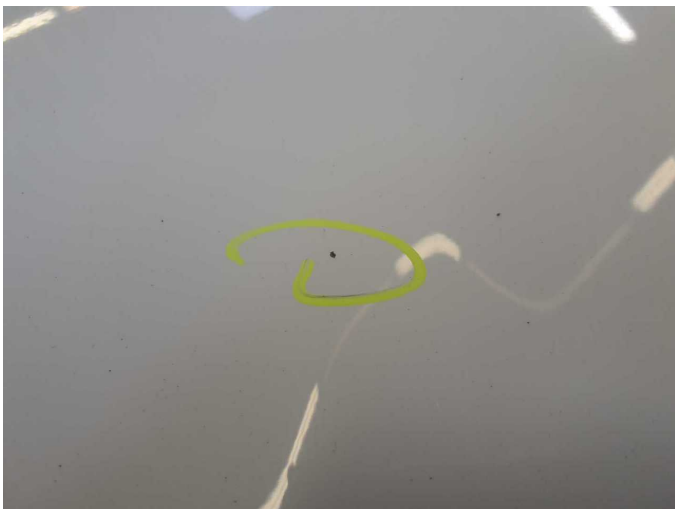
Damage 10: Bonnet: Bonnet - Stone chips - Paint
