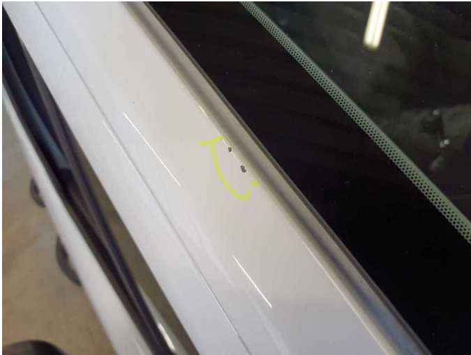
Damage 4: Roof: Roof rail - right side - Stone chips - Smart repair
