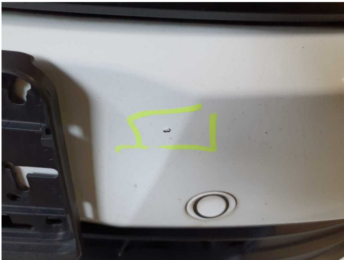
Damage 11: Front bumper: Front bumper - Scratched - Paint
