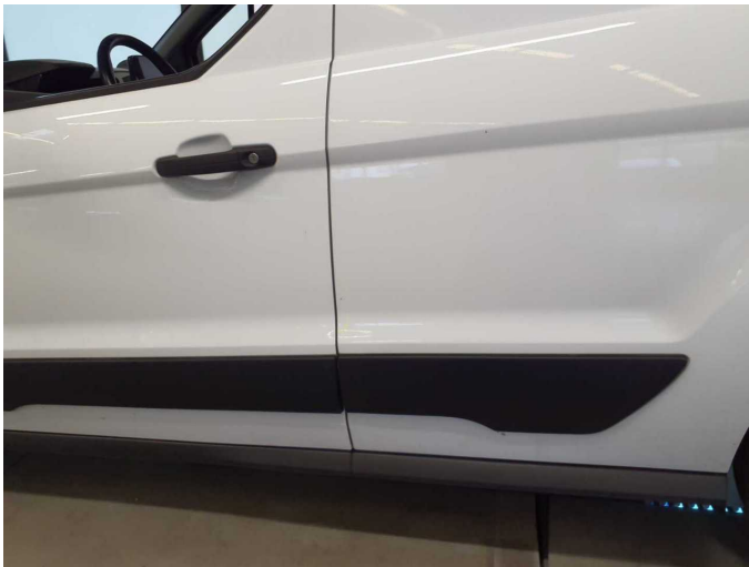
Damage 5: Side panel - rear left side: Side panel - Scratched - Smart repair
