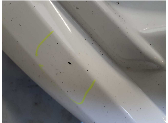
Damage 11: Front bumper: Front bumper - Scratched - Paint
