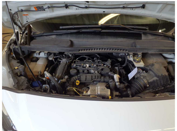
Missing part 2: Engine: Engine cover - Missing - Replace
