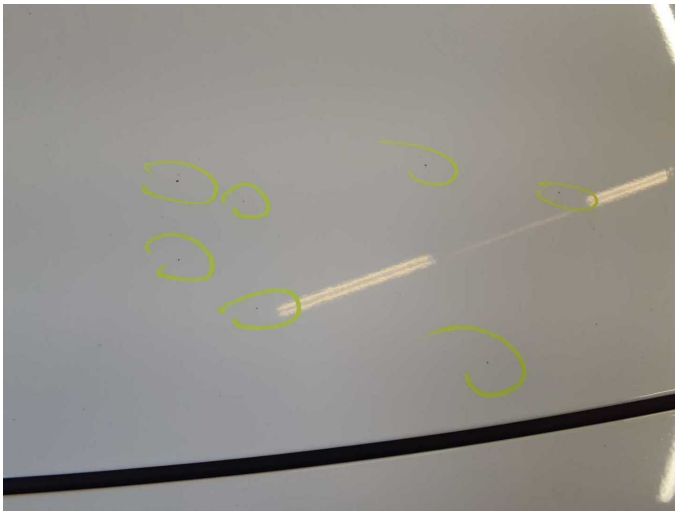
Damage 10: Bonnet: Bonnet - Stone chips - Paint
