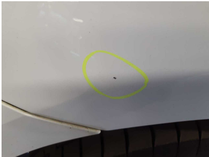
Wear and tear 3: Mudguard - left side: Wheel arch - Stone chips - No deduction
