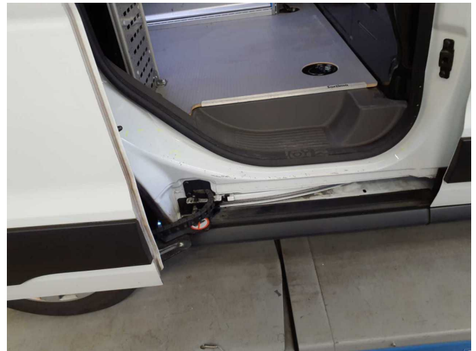
Damage 7: Sill - right side: Cat walk - Dent / paintcoat damage - Smart repair
