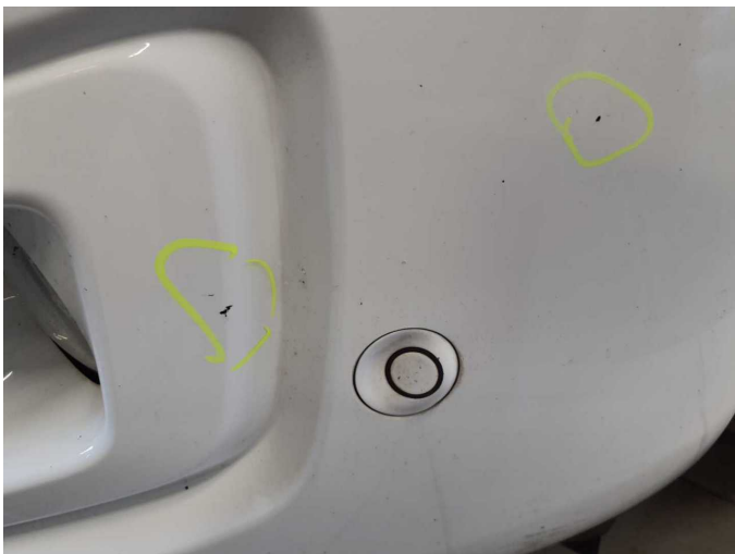
Damage 11: Front bumper: Front bumper - Scratched - Paint
