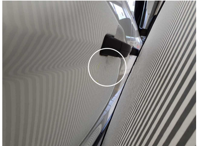
Wear and tear 6: Sliding door, right: Sliding door (außen) - dent(s) - No deduction
