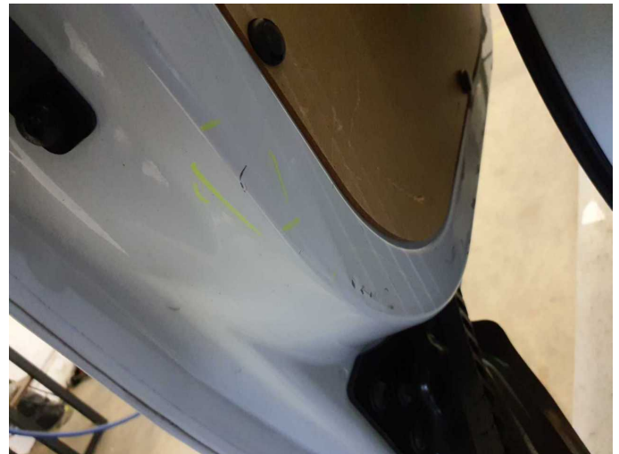
Damage 3: Sliding door, right: Sliding door (innen) - Dent / paintcoat damage - Smart repair
