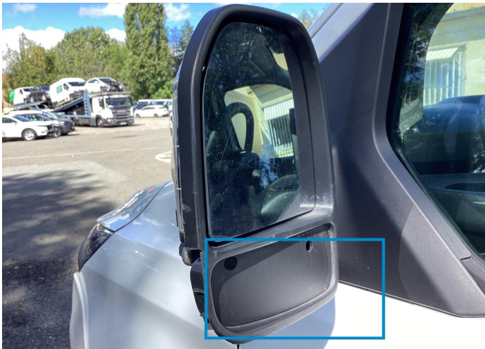
18. Mirror Glass / Front Left Missing Part -
