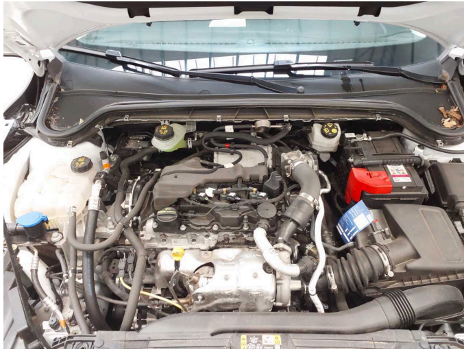
Damage 1: Engine: Engine cover - top / cover - Missing - Replace
