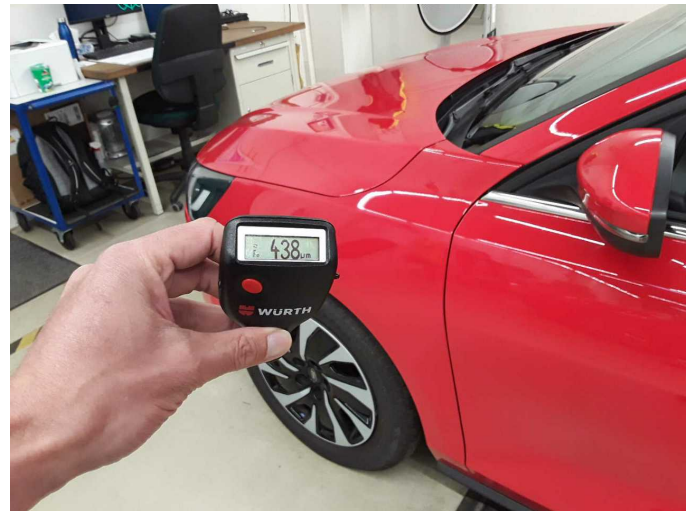
Mudguard - left side: 438 µm
