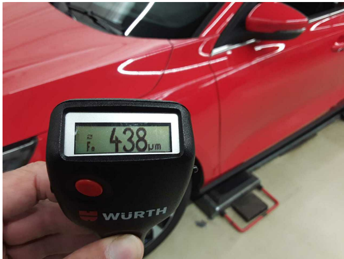
Mudguard - left side: 438 µm
