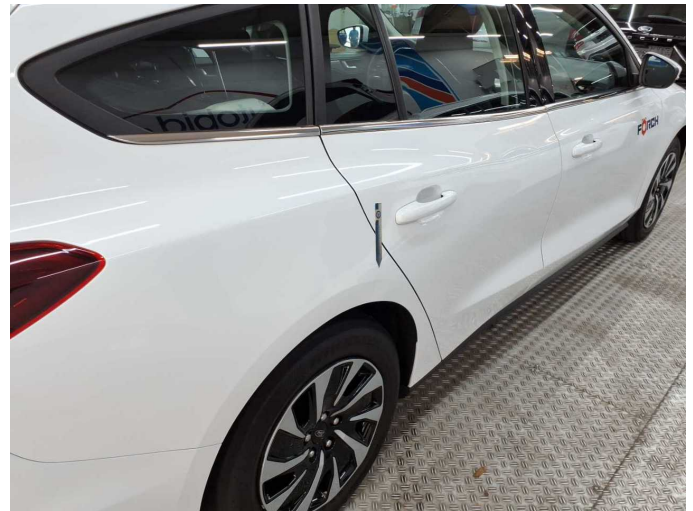
Damage 3: Side panel - rear right side: Side panel (Kante) - dent(s) - Smart repair
