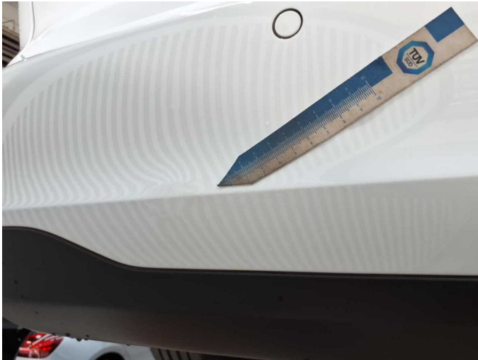
Damage 4: Rear bumper: Rear bumper (Kante) - dent(s) - Repair and paint
