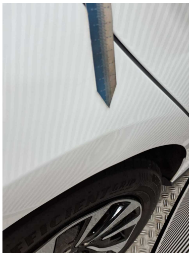
Damage 3: Side panel - rear right side: Side panel (Kante) - dent(s) - Smart repair
