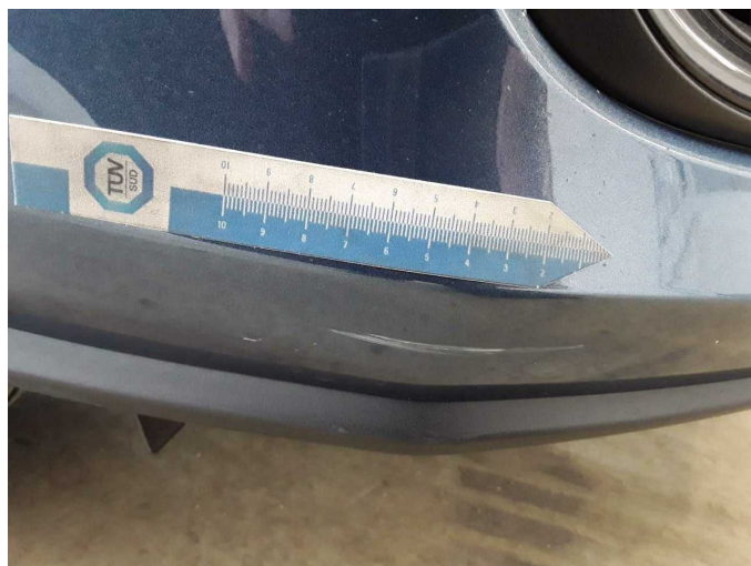
Damage 5: Front bumper: Front bumper - Scratched - Paint
