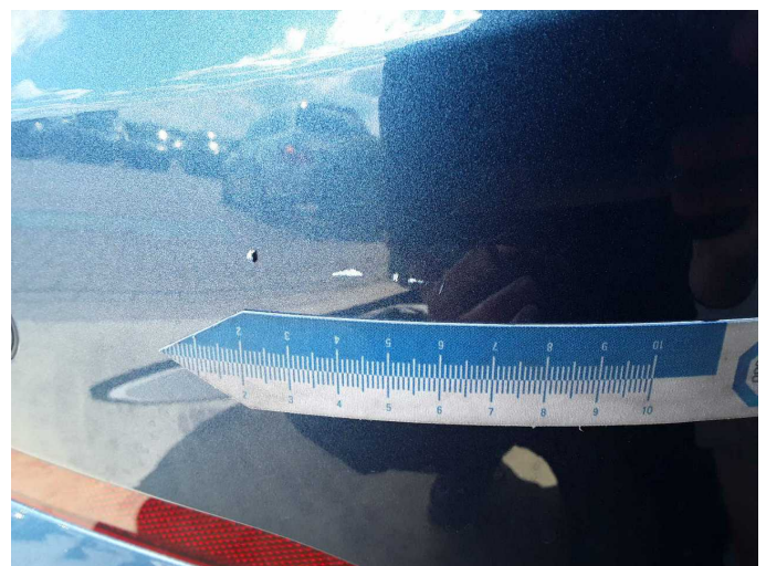
Damage 4: Rear bumper: Rear bumper - Scratched - Paint
