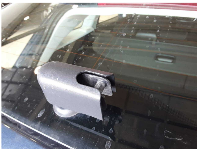
Damage 1: Screen cleaning: Wiper arm - rear - Broken / torn - Replace
