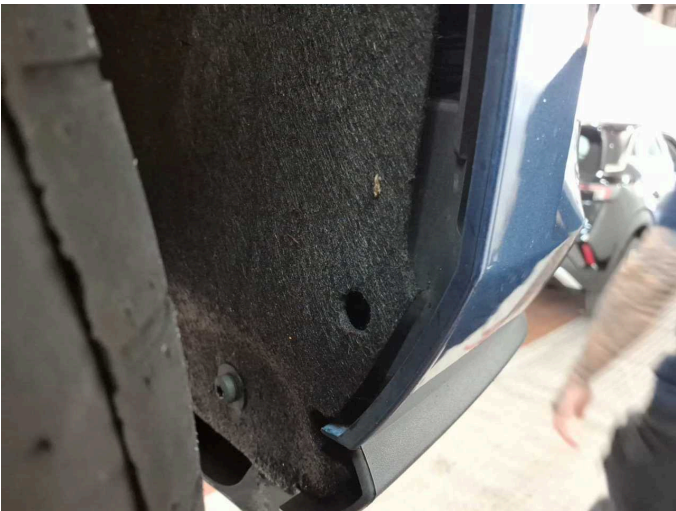
Damage 1: Body: Wheel well - front right side (Klip fehlt) - Missing - Replace
