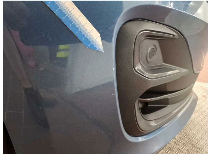
Damage 3: Front bumper: Front bumper - Scratched - Paint
