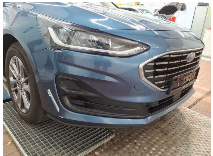
Damage 3: Front bumper: Front bumper - Scratched - Paint
