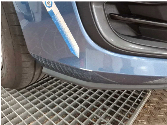
Damage 3: Front bumper: Front bumper - Scratched - Paint
