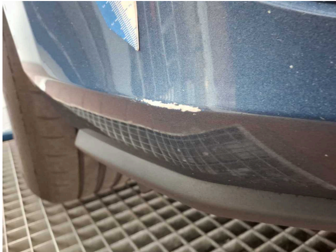
Damage 3: Front bumper: Front bumper - Scratched - Paint
