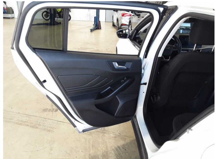
Damage 3: Trim / covers: Door trim - rear left side - Scratched - Replace
