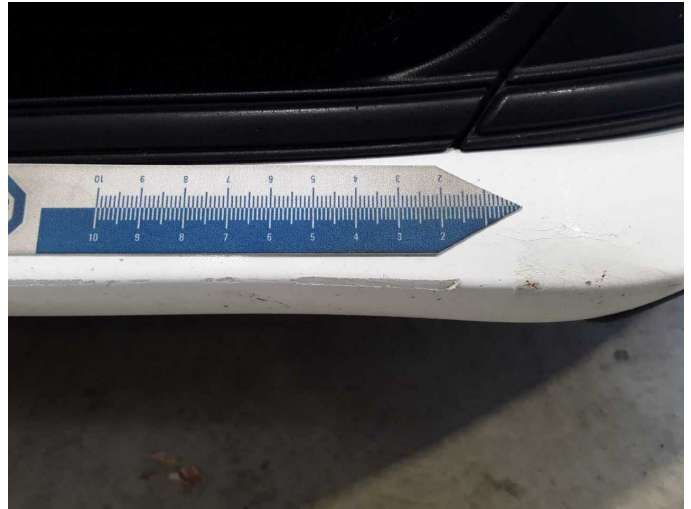
Damage 4: Front bumper: Front bumper - Scratched - Paint
