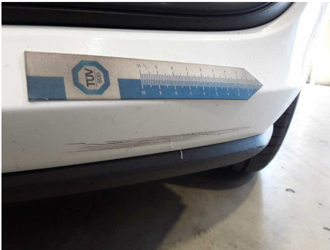
Damage 4: Front bumper: Front bumper - Scratched - Paint
