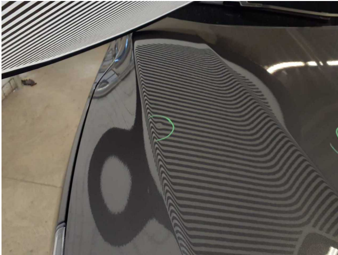
Damage 5: Bonnet: Bonnet - dent(s) - Smooth repair work
