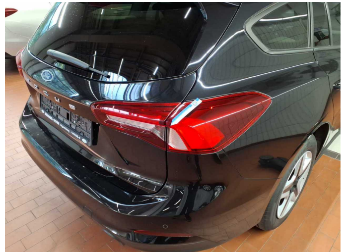
Damage 5: Tail light: Tail lamp - right side - Scratched - Replace
