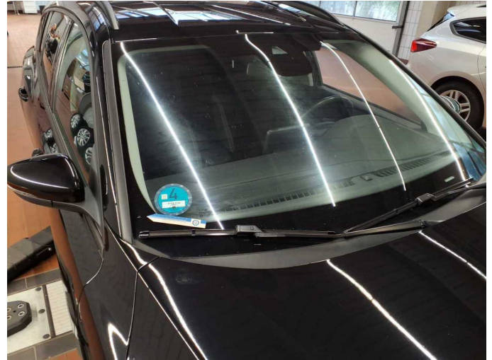
Damage 9: Vehicle glazing: Windscreen - Stone chips - Replace
