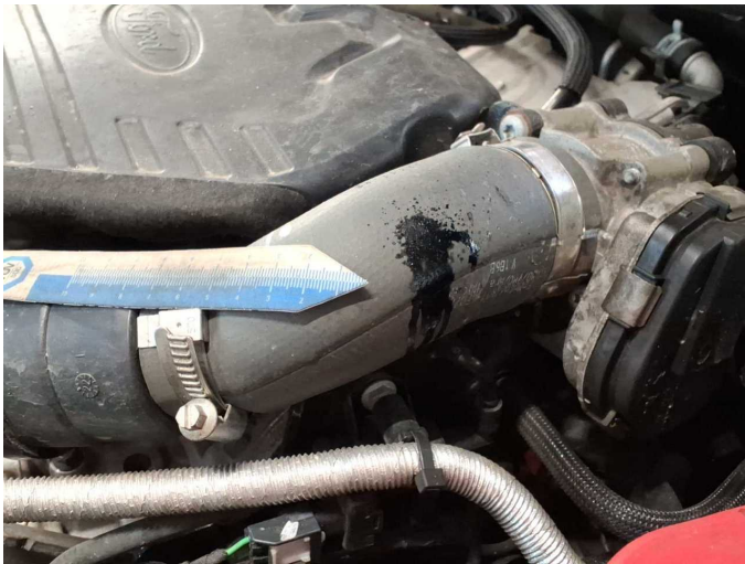
Damage 1: Engine: Hose turbocharger (Mehrkosten möglich) - Damage caused by marten / rodent - Replace
