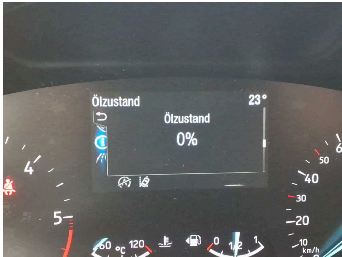
Damage 5: Misc.: Inspection / maintenance - Due - Perform
