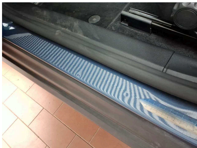
Damage 3: Sill - left side: Sill (2 Dellen) - dent(s) - Smart repair
