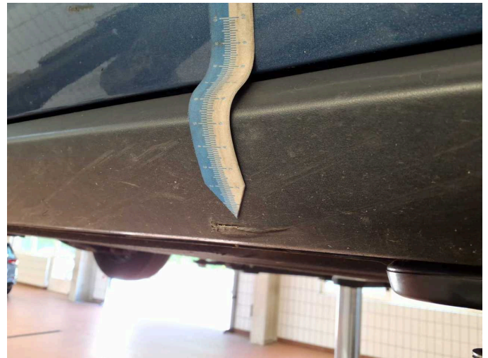
Damage 6: Sill - right side: Trim - Broken / torn - Replace
