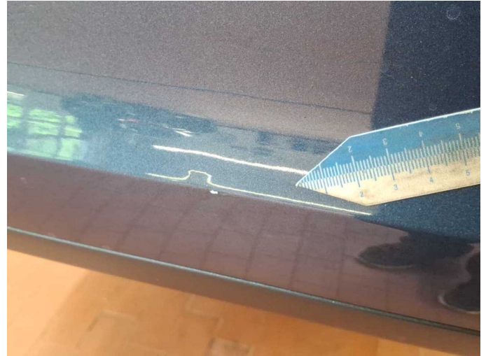
Damage 8: Rear bumper: Rear bumper - Scratched - Paint
