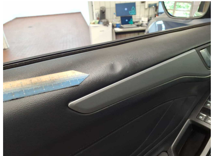
Damage 4: Trim / covers: Door trim - front left side - dent(s) - Smart repair
