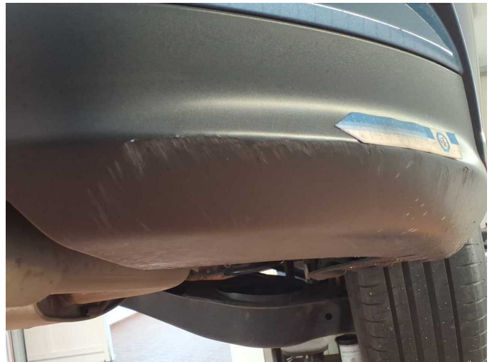
Damage 7: Rear bumper: Spoiler - Scratched - Replace
