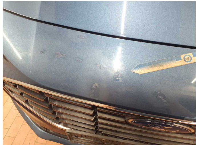
Damage 9: Front bumper: Front bumper - Scratched - Paint
