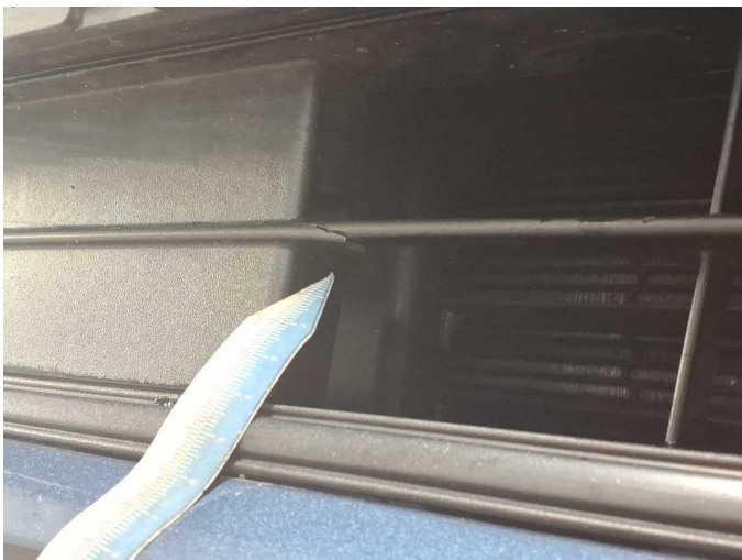
Damage 2: Front bumper: Air-inlet grille - Broken / torn - Replace
