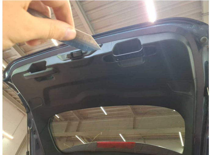
Damage 6: Trim / covers: Boot lid - interior trim - Damaged - Replace
