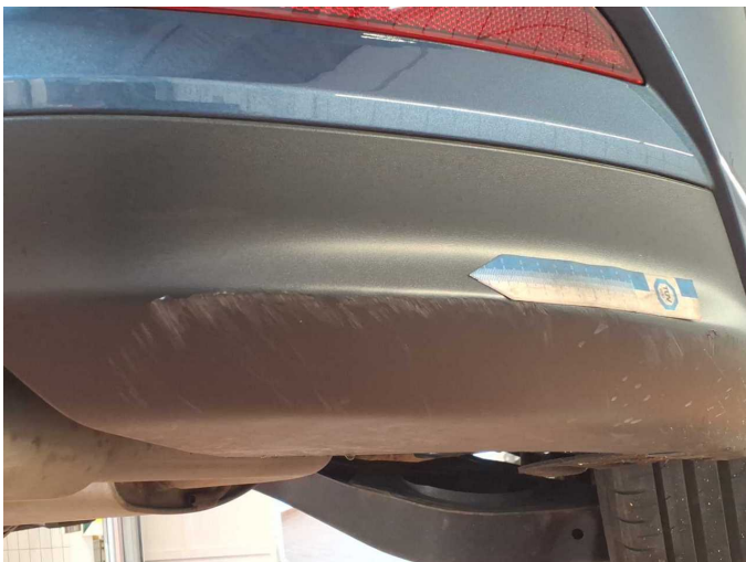
Damage 7: Rear bumper: Spoiler - Scratched - Replace
