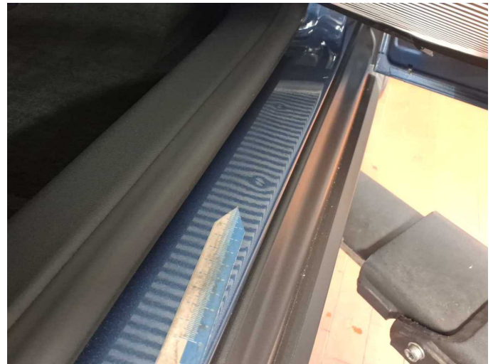
Damage 3: Sill - right side: Sill (2 Dellen) - dent(s) - Smart repair
