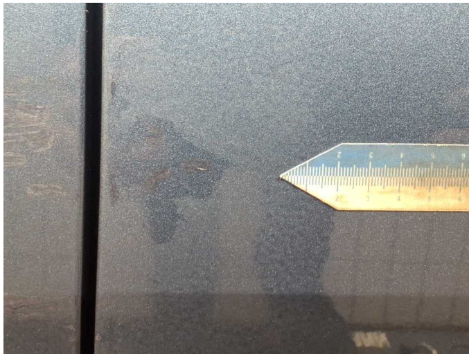
Damage 11: Door - front right side: Door - Scratched - Paint
