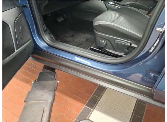
Damage 1: Sill - left side: Sill - dent(s) - Smart repair
