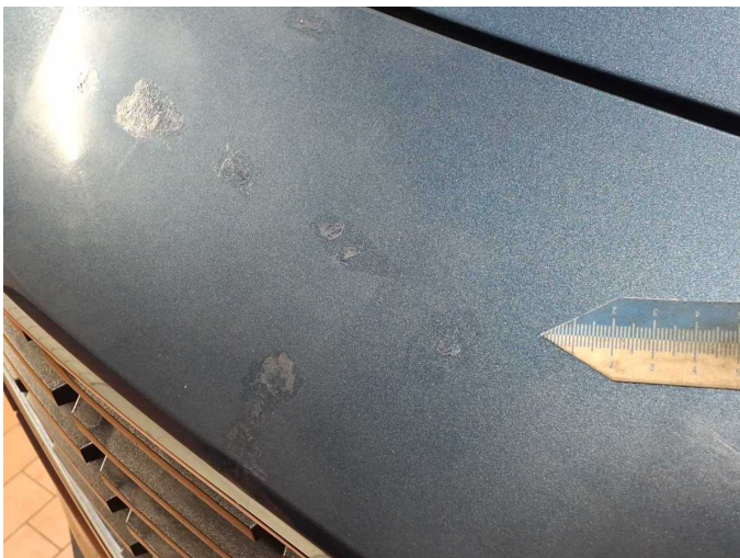
Damage 9: Front bumper: Front bumper - Scratched - Paint
