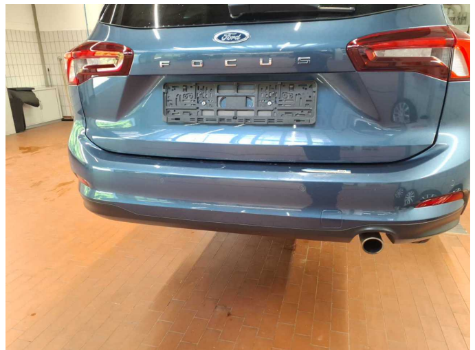
Damage 8: Rear bumper: Rear bumper - Scratched - Paint
