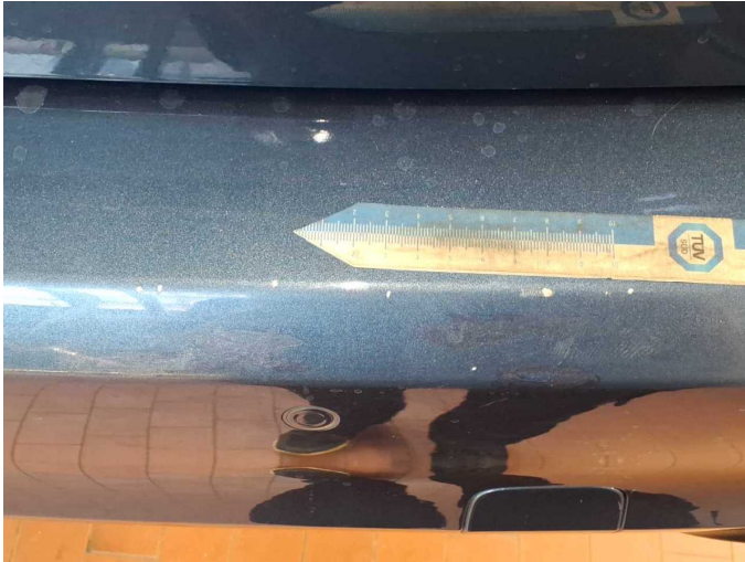
Damage 8: Rear bumper: Rear bumper - Scratched - Paint
