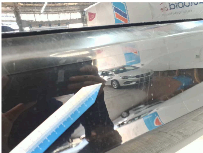
Damage 3: Rear bumper: Rear bumper - Scratched - Replace
