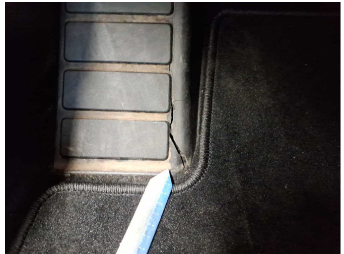
Damage 1: Trim / covers: Floor covering - front left side (Fußablage links) - Broken / torn - Replace
