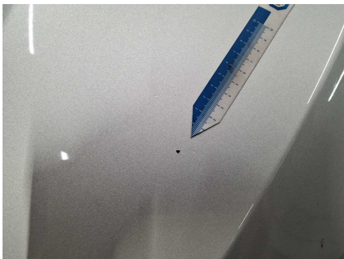
Damage 10: Bonnet: Bonnet - Stone chips - Paint
