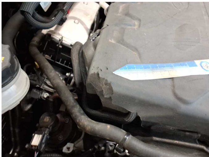
Damage 9: Engine: Engine (Abdeckung, Schlauch) - Damage caused by marten / rodent - Replace
