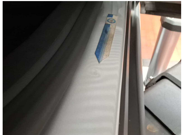
Damage 4: Side panel - rear right side: Sill - dent(s) - Smart repair
