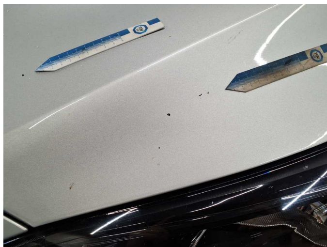
Damage 10: Bonnet: Bonnet - Stone chips - Paint
