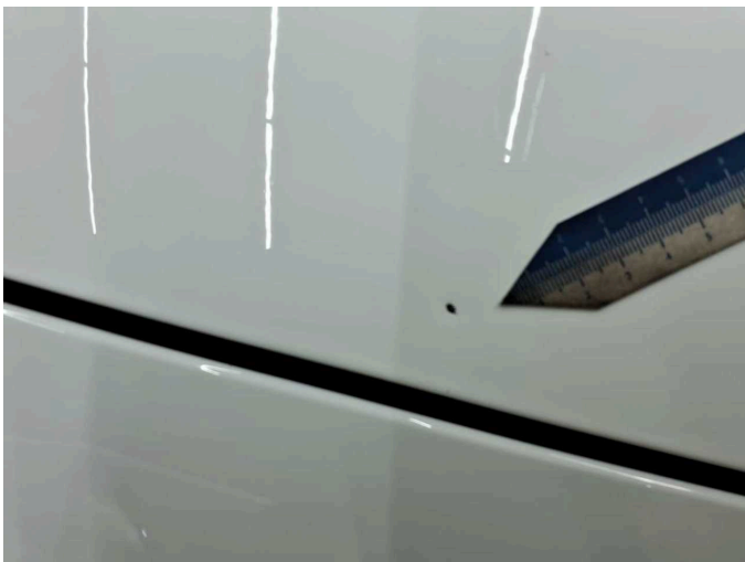
Damage 6: Bonnet: Bonnet - Dent / paintcoat damage - Paint
