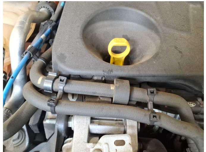
Damage 7: Engine: Engine cover - top / cover - Damage caused by marten / rodent - Replace
