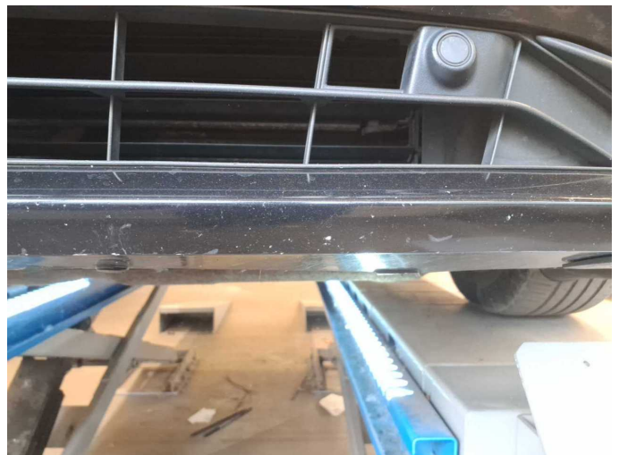
Damage 11: Front bumper: Front bumper - Scratch(es) - Paint
