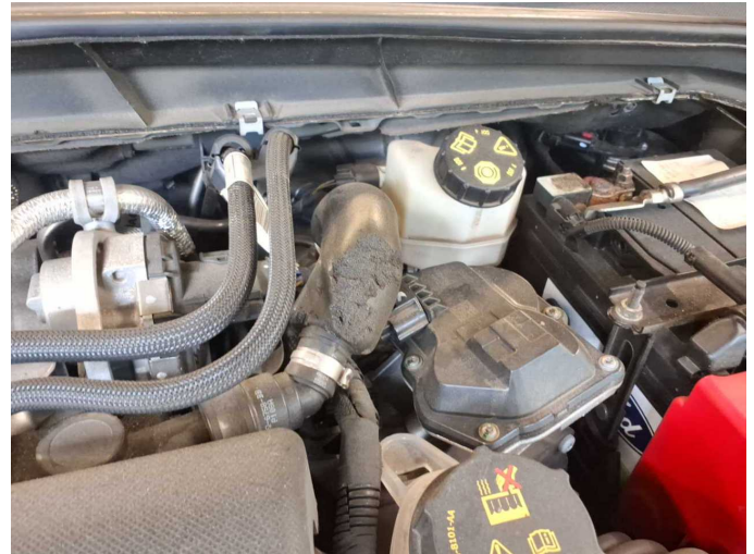
Damage 2: Engine: Engine (Rohr Ölabscheider) - Damage caused by marten / rodent - Replace
