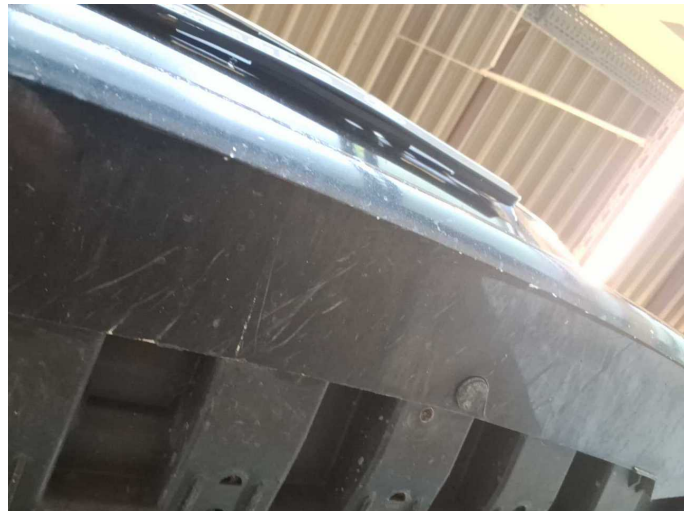
Damage 11: Front bumper: Front bumper - Scratch(es) - Paint
