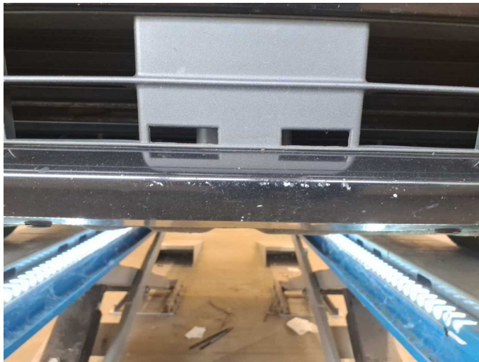
Damage 11: Front bumper: Front bumper - Scratch(es) - Paint
