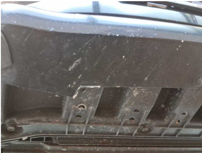
Damage 11: Front bumper: Front bumper - Scratch(es) - Paint
