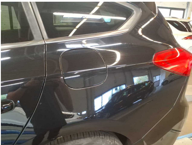
Damage 1: Fuel system: Tank flap - Scratch(es) - Smart repair
