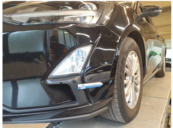
Damage 11: Front bumper: Front bumper - Scratch(es) - Paint
