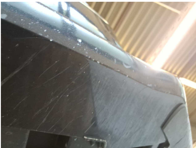
Damage 11: Front bumper: Front bumper - Scratch(es) - Paint
