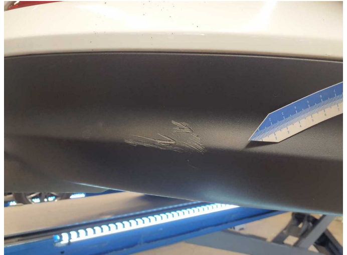
Damage 3: Rear bumper: Spoiler - Scratch(es) - Replace
