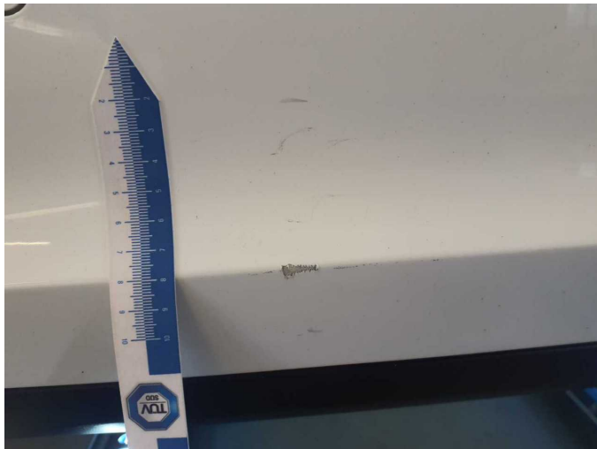
Damage 4: Rear bumper: Rear bumper - Scratch(es) - Paint
