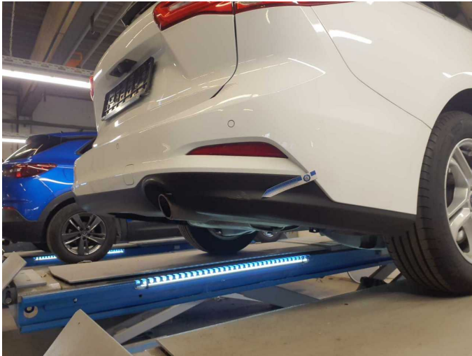
Damage 3: Rear bumper: Spoiler - Scratch(es) - Replace
