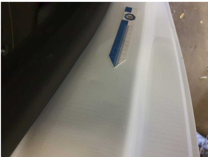
Damage 2: Side panel - rear right side: Sill (2) - dent(s) - Smart repair
