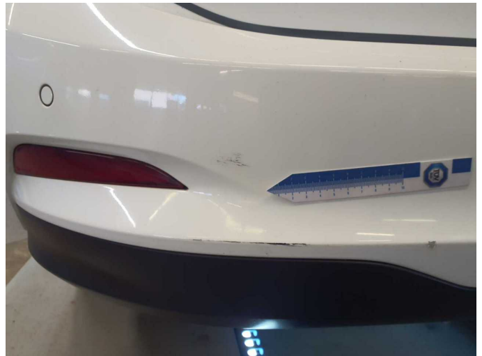
Damage 4: Rear bumper: Rear bumper - Scratch(es) - Paint
