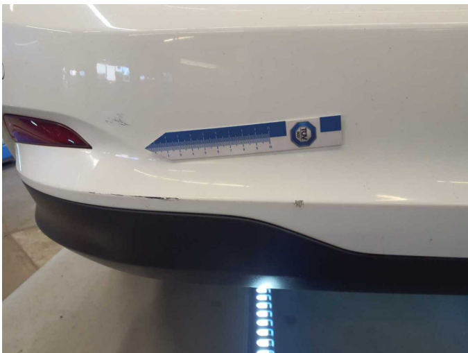
Damage 4: Rear bumper: Rear bumper - Scratch(es) - Paint
