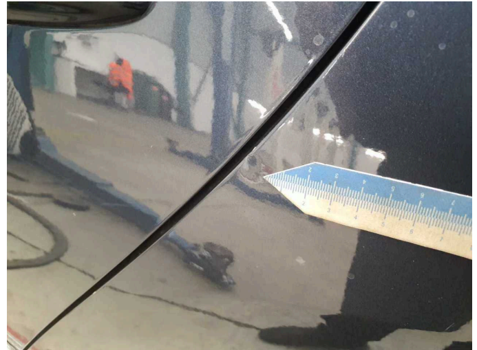
Damage 3: Side panel - rear left side: Side panel - Dent / paintcoat damage - Repair and paint
