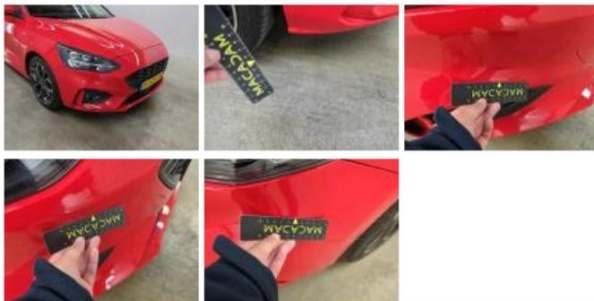
Door RR, Dent(s), Repair and paint (complete)
