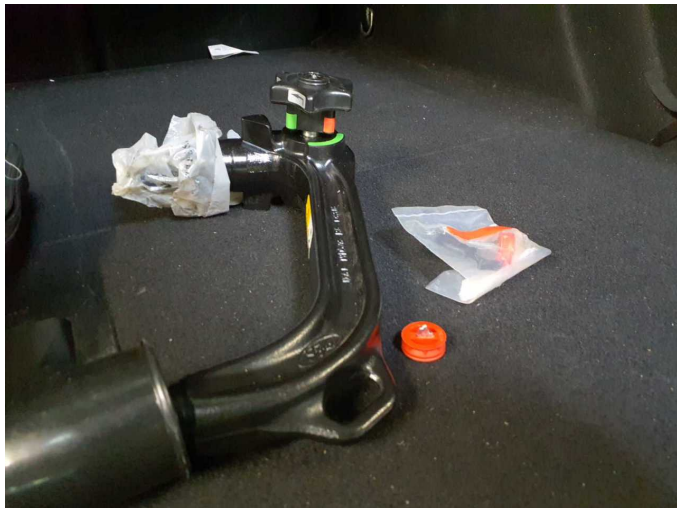
Damage 1: Rear of vehicle: Key trailer hitch - Broken / torn - Replace
