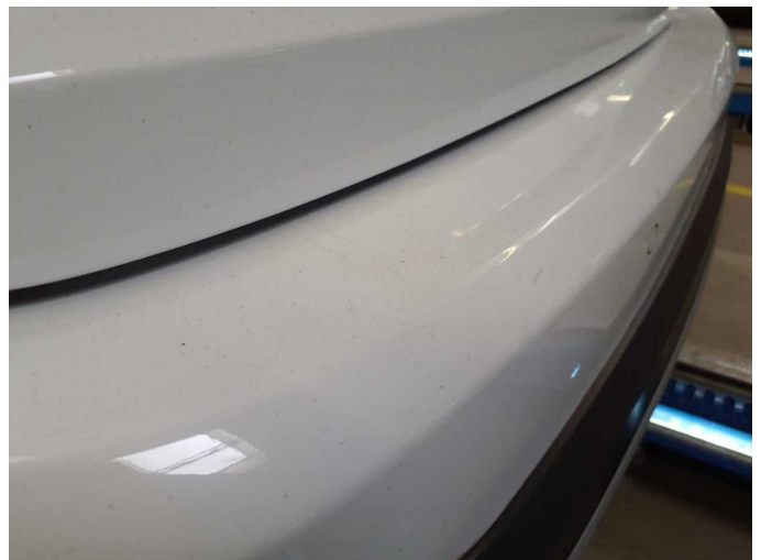
Damage 7: Body: Body - Soiled - Conditioning
