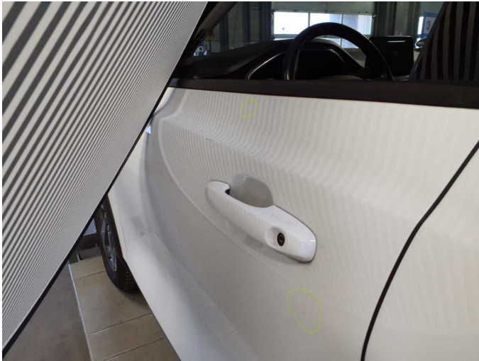
Damage 12: Body: Body - Damage by hail - repair according to calculation
