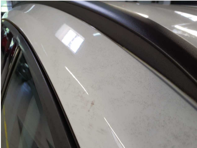
Damage 7: Body: Body - Soiled - Conditioning
