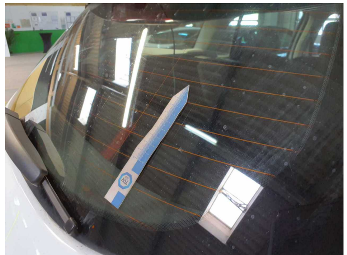
Wear and tear 8: Vehicle glazing: Rear window - Scratched - No deduction
