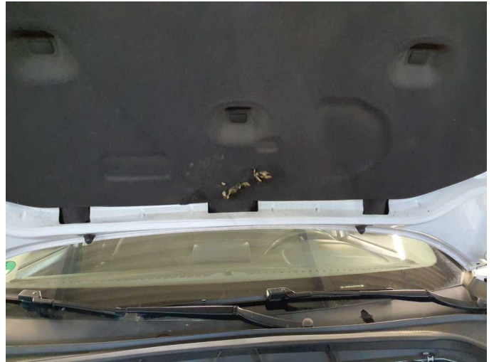
Damage 6: Bonnet: Insulation lining - Holes - Replace
