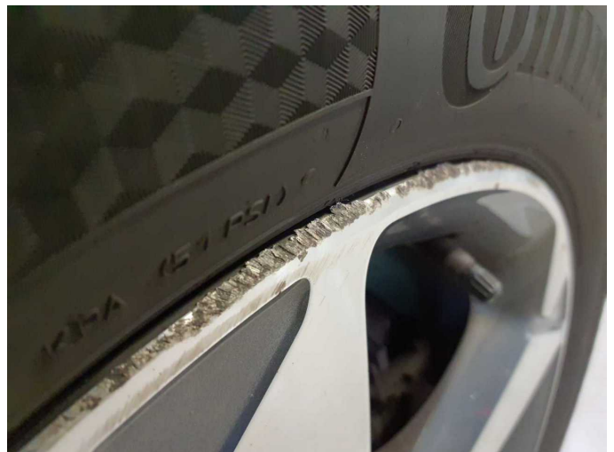
Damage 8: Wheel / tyres: Alloy rim - rear left side (Materialabtrag) - Damaged - Replace
