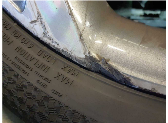
Damage 9: Wheel / tyres: Alloy rim - front left side (Materialabtrag) - Damaged - Replace
