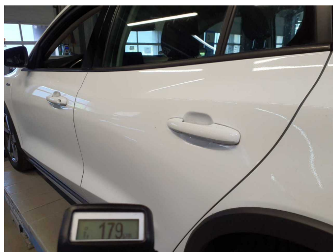
Repainting 5: Door - rear left side
