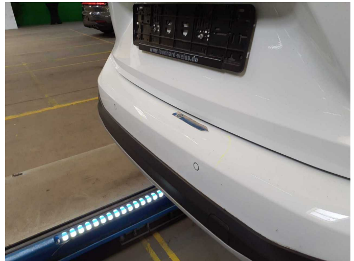
Damage 10: Rear bumper: Rear bumper (verformt) - Scratched - Repair and paint
