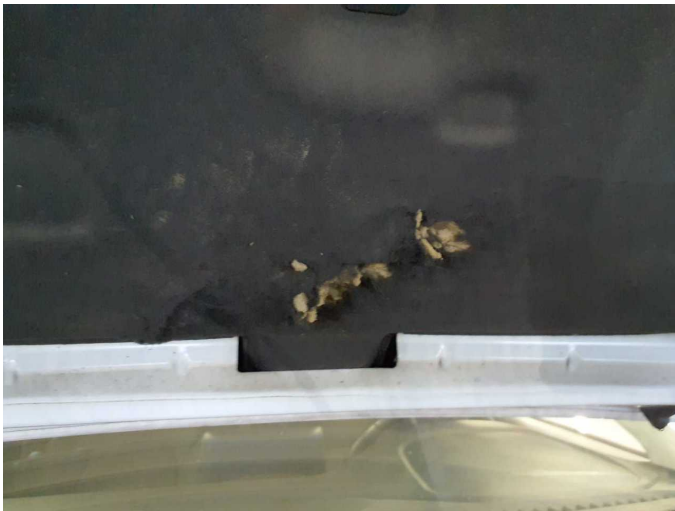
Damage 6: Bonnet: Insulation lining - Holes - Replace
