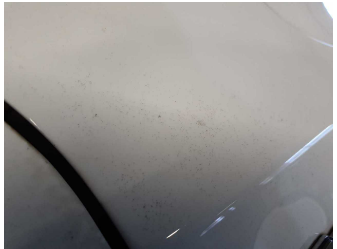
Damage 7: Body: Body - Soiled - Conditioning
