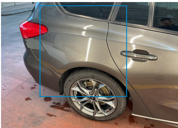
5. Fender / Back Right Bodywork / Poor Previous Repair -
