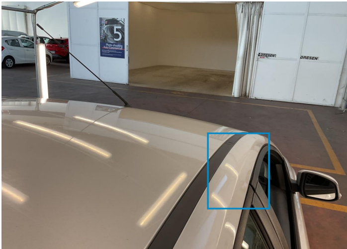
25. Pillar / Front Right Bodywork / Dent -
