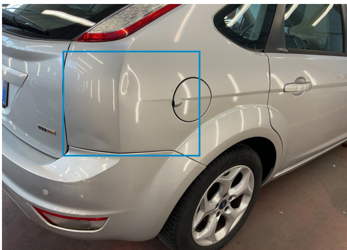
17. Fender / Back Right Bodywork / Dent -
