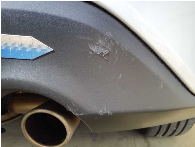
Damage 2: Rear bumper: Spoiler - Scratch(es) - Replace
