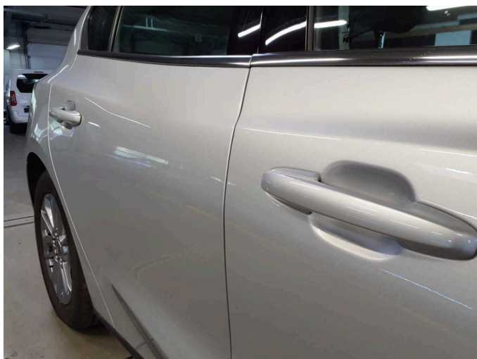
Wear and tear 5: Door - front right side: Door handle - outside - Scratched - Cover / polish
